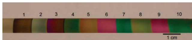
Figure 2. Photograph of a series of ZIF-8 films of various thicknesses grown on silicon substrates.
